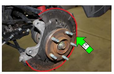
20. Bolt the purple brackets (silver in this picture) (14-56250) into place using the hex head bolts (36-10442), as shown (15). Use blue Loctite and torque them to 33 ft-lb. The rear brackets are identical from side to side, but make sure they're installed as shown. "Flyin' Miata" should be visible from the inside, as with the fronts.
