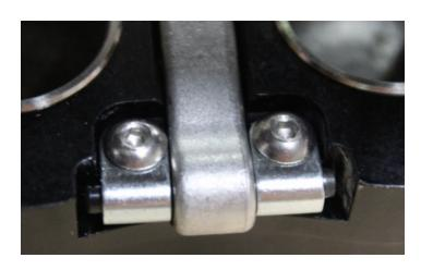
23. Bolt the calipers into place, using the rounded-head (36-10780) Allen key bolts (16). Again, use blue Loctite and tighten to 33 lb-ft.
