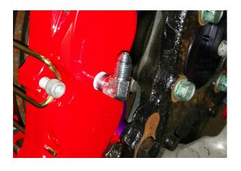
10. Thread the brake line (14-66110) onto the fitting installed in step 8. Orient it so that the natural curve of the brake line orients it nicely with the stock hard line, then get the fitting finger tight. Use a wrench to turn it a 1/4 turn farther. Temporarily install the wheel and check to make sure that the brake line can't contact the wheel at any steering angle.
