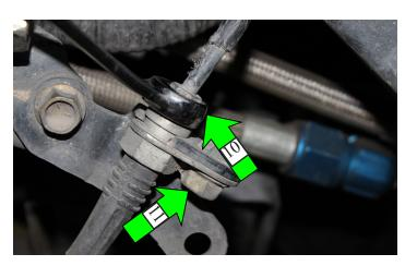
12. Slip the new hose into the bracket, and line it up with the fitting. Get the stock fitting threaded finger-tight (or something close), then reinstall the bolt (11). Tighten the stock fitting to 10 - 16 ft-lb.
