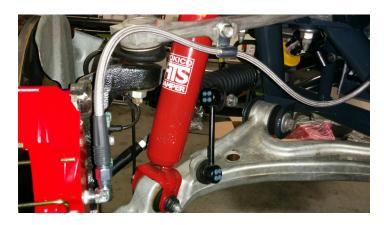
11. Using a 10mm flare wrench, loosen the fitting on the stock hard line where it attaches to the stock rubber soft line (10). Be very careful not to strip the hex on the fitting - this is especially true if you're not using a flare wrench. This junction will drip brake fluid, but it won't pour out. Remove the bolt (11), then slip the rubber hose out.
