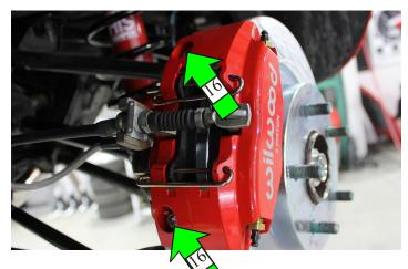
24. Smear a little thread sealant on the fitting that threads into the caliper (don't get any on the first two threads). Thread the fitting (included with 14-66220) into the caliper until it's finger tight, then go 1.5 - 3 turns farther. These are tapered threads, so don't expect it to visibly bottom out on anything (the fitting in the picture is tight). Don't overtorque! (The brake line shouldn't be installed yet.)
