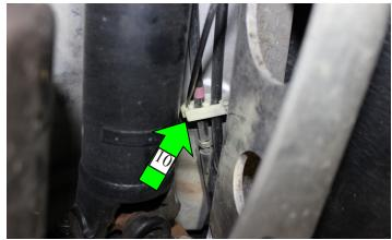
16. Remove the parking brake cable from the the backside of the caliper. Remove the metal clip (11), then pull the housing away from the caliper to disengage it from its hole. Then, pull the cable toward the caliper and rotate it down to unhook the cable end (12) from the caliper. Pull the cable out so that it hangs underneath the fuel tank. Leave it here for the time being.
