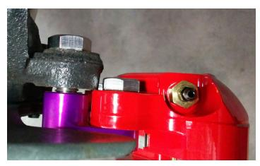
the center of the hub). Then remove the caliper assembly. In the axial direction (towards the center of the car), you'll need to take about 1/8" (3mm) off, as shown (4). It's typically easiest to do this with a cutoff wheel (which are often about 1/8" thick). A hacksaw or grinder could also be used. Some trial and error may be required, but with some patience and the right tools, it's not too hard.
