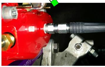
25. Thread the brake line (14-66220) onto the fitting installed in step 20. No thread sealant should be used here. Orient it so that the natural curve of the line lines it up nicely with the stock hard line, then get the fitting finger tight. Then use a wrench to turn it a 1/4 turn farther. (The hose shouldn't be connected to the stock hard line yet, nor should the parking brake cable be installed.)
