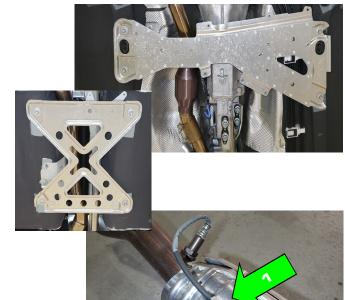
5. Locate the flange where the mid-pipe is secured to the exhaust manifold. Using a 14mm socket or wrench, loosen the two nuts. To keep the pipe from accidentally falling, don't fully remove either nut until both ends of the pipe are loose and you're ready to remove it.
